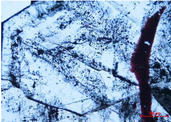
Fig. 1. Euhedral crystal of the first quartz generation (Qz I) with distinctive growth zones containing primary fluid inclusions.
